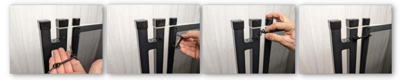
Screw the Eye into the Gate Truss. (A small screwdriver will help turn the eye to thread it into the truss). Then screw the Section Latch into the pole and connect the two. At this point you will remove (cut) the zip tie.
