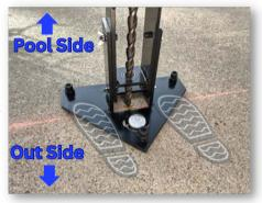
Adjusting the three Allen bolts up or down on the base of the Drill Guide will allow you to level the guide. You will know it is level when the bubble is in the middle circle.
