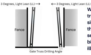
When drilling the gate truss, turn the drill guide sideways and drill on the Light Lean (LL) selection. Align the drill bit on your mark as illustrated below
