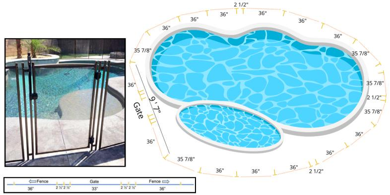
On your chalk line, make two "T" marks 33" apart and then two more at 2 1/2" out from your original marks. This will be your Double Pole Gate Truss for your gate. From your original gate truss marks, measure and mark "T" at 2 ½". This will be the first pole in the section of fence. Continuing on your straight chalk line, mark 36" from your 2 1/2" mark.
